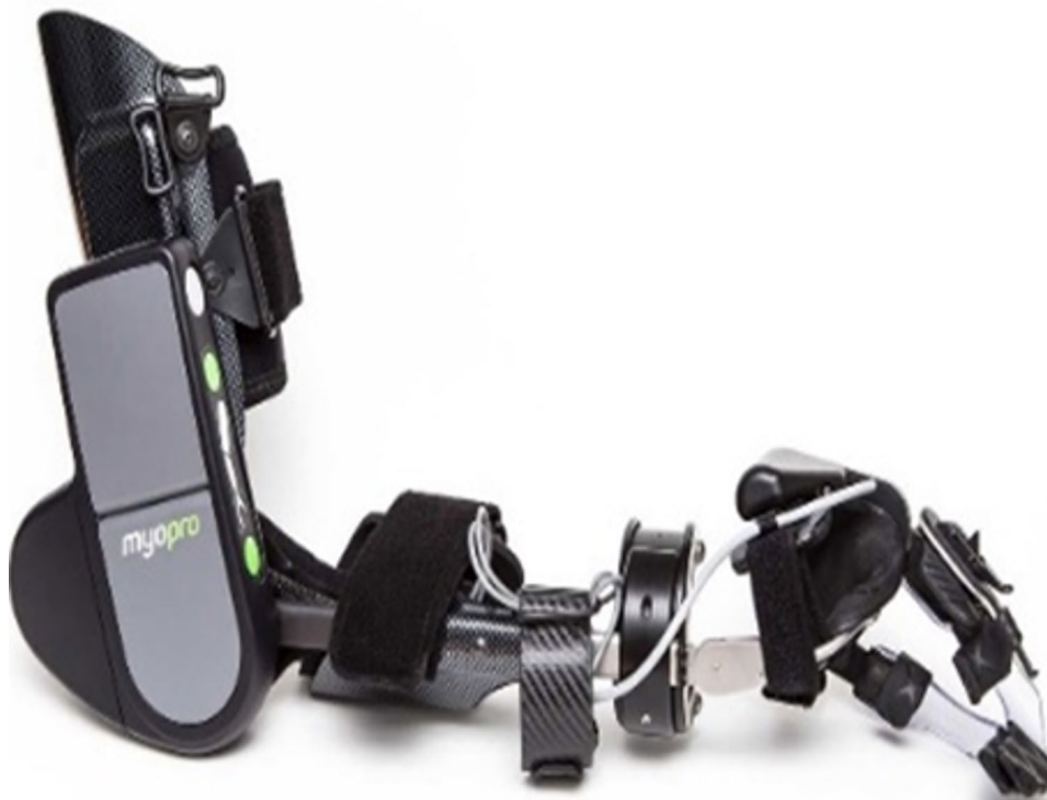
Fig. 2 Illustration of the myoelectric upper extremity MyoPro MPWO
