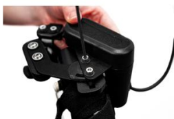
6. Tighten screws above the motor to secure Palmer Grip in place.
