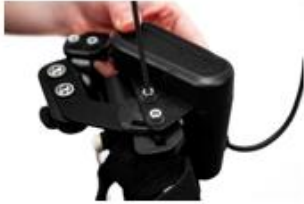
2. Flip hand piece over and loosen screws above the motor. Do not completely remove the screw.
