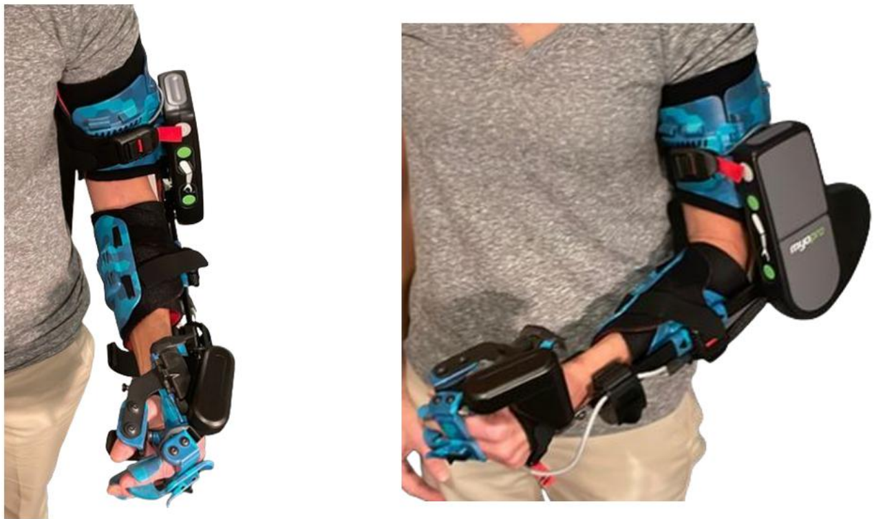
13 Close the humeral shell lining, shell, and then magnetic clasp
