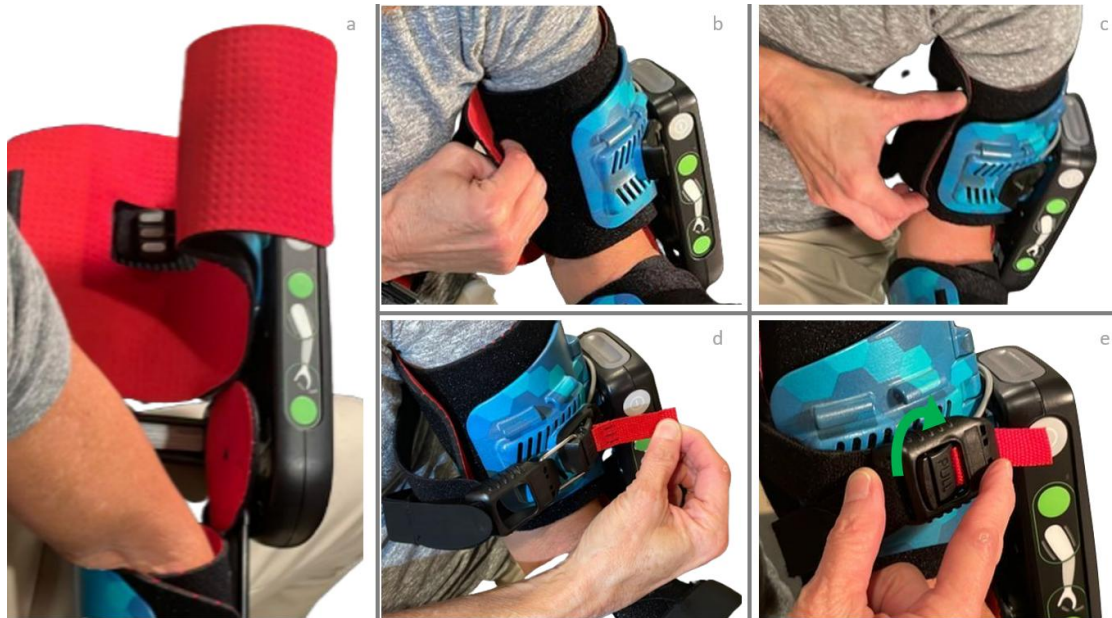
13 Close the humeral shell lining, shell, and then magnetic clasp
