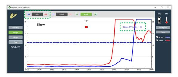
The number beside the gain header [image above, top left] represents the amount of amplification used for that mode. The numbers are color coded to coincide with the mode, e.g. the blue number next to the gain button represents the gain for the biceps mode that correlates to the elbow of the MyoPro bending.
