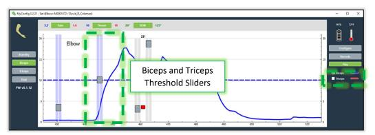
Since the device in the preceding photo is in *Biceps* mode, only the biceps EMG is being graphed. Additionally, only the biceps *threshold* is visible to indicate that the device is only responding to the biceps EMG in this mode.
