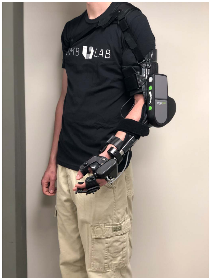
Figure 1. Patient with a left brachial plexus injury with inadequate elbow flexion with a MyoPro G device (Myomo, Inc, Cambridge, MA).
